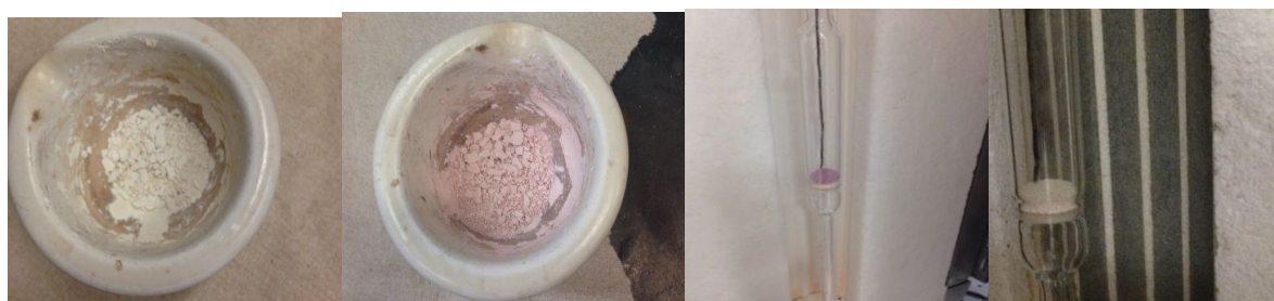
Figure S5. Visual changes to 1 wt% Pd/SSZ-13 with Si/Al ratio 6 single-atom material: a). in the presence of moisture b). dehydrated under helium or oxygen (note that these changes are reversible; when the pink sample is stored in the glove box in the absence of moisture it retains its colour; as soon as water is added in the glovebox or the sample is taken out of the glovebox, the colour changes to yellowish) c). Pd/SSZ-13 exposed to CO d). Pd(II)(CO) _2 /SSZ-13 exposed to a single pulse of ethylene with the formation of classical colourless (in the VIS region) Pd(II)(CO)(C _2 H _4 ) complex.
